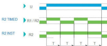
Function Di - Symmetrical flashing (ON Start)
