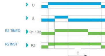
Function C - Off-Delay (Delay on break)
