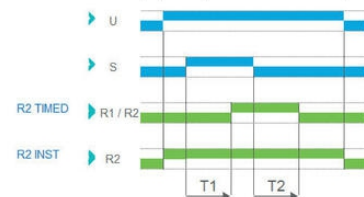
Function Ac - On/Off Delay (Delay on make/break)
