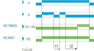
Function At - Summation time relay
