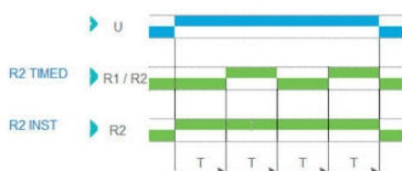
Function D - Symmetrical flashing (OFF Start)
